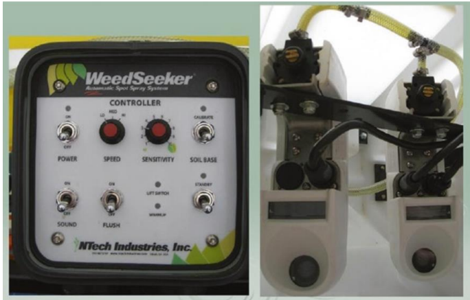
Weed seeker, controller, and sensors
